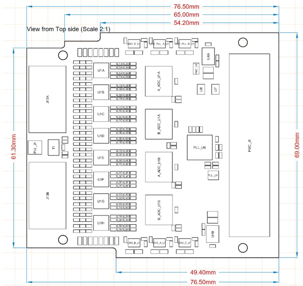
Figure 3 - SMT-FMC116 Components Placement – Prototype
