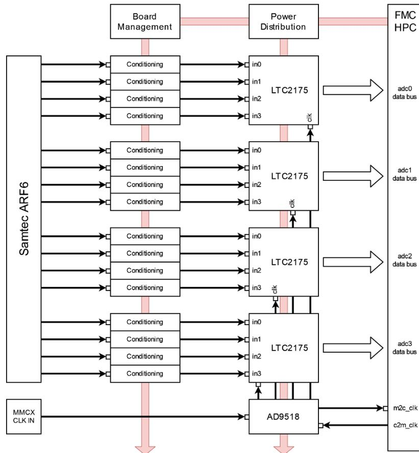
Figure 1 General Block Diagram of SMT-FMC116
